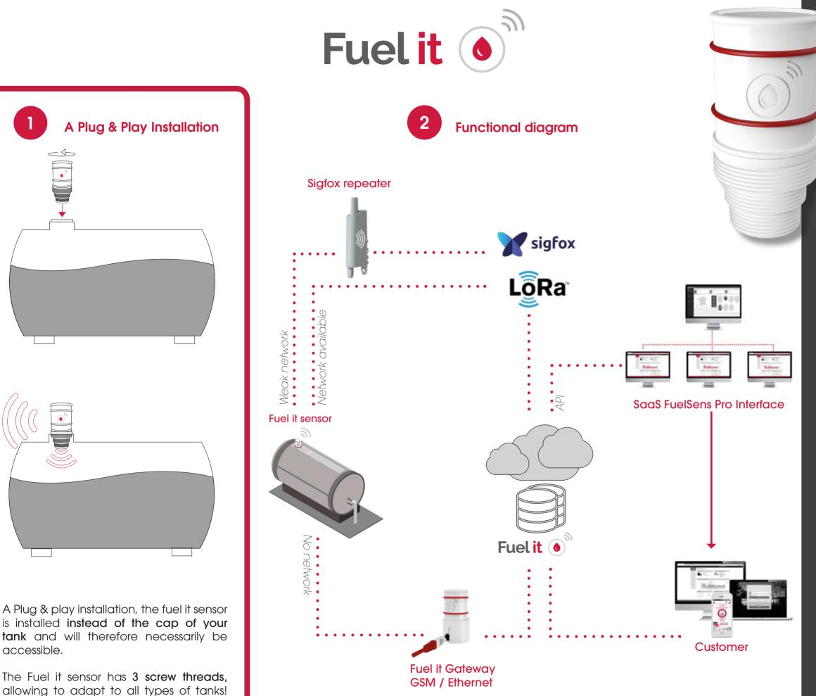
allowing to adapt to all types of tanks! Its installation is easy, to activate it you must pass the magnet (supplied in the packaging) near the sensor; a blue light appears: the installation is successfully completed!
